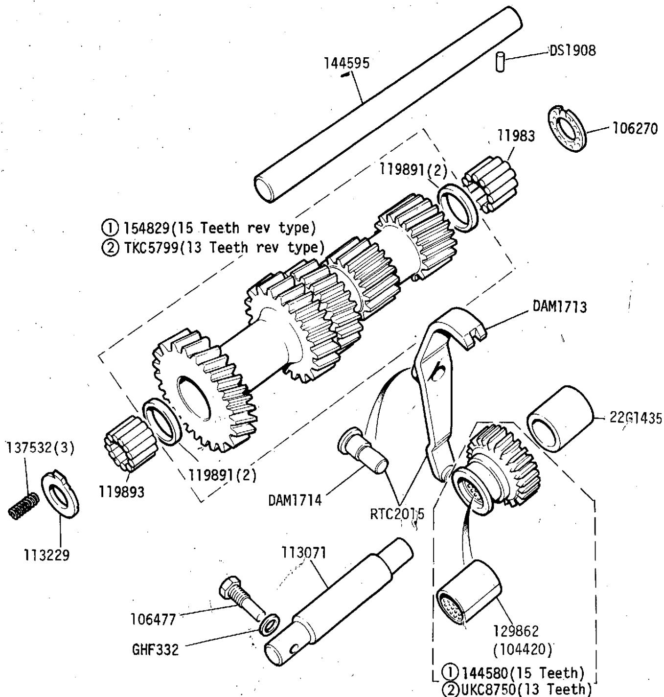
① Parts of gearbox assemblies UKC5643 and UKC5646
